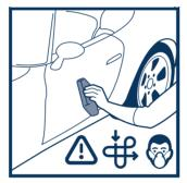
Apply a thick layer of Q2 FLASH EVO. Level the apply a thick layer of Q<sup>2</sup> FLASH EVO. Level the coating well. Apply in your preferred motion. Levelling is crucial, not the application pattern. We recommend applying full panels. Split panels only while applying at high temperature or humidity.
