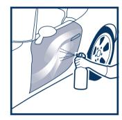
Ensure the surface is oil-free and completely dry. Use of  ${\sf Q}^2{\sf M}$  PREP is obligatory.
