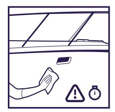
The maximum size of the section depends on temperature and humidity. Wipe of immediatelly after the coating has been applied to a section. Do not allow to dry.
