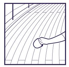
Apply a moderate amount of product in straight line motion. Ensure an even finish, as wipe off is not necessary. Rub the product in the surface.
