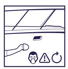
Apply a thick layer of  $Q^2R$  GelCoat in circular motion with the attached applicator. Pay attention to the leveling of the coating.
