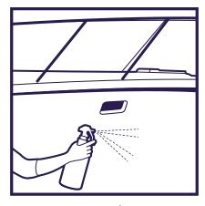
Prepare the surface with  $Q^2R$  Degrease. Use a moderate amount of product and wipe with a microfibre. Ensure the surface is oil free and completely dry.
