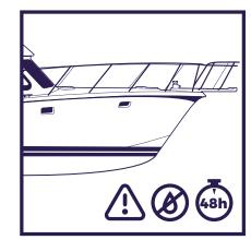
Let the coating cure for 48 hours. Avoid any contact with water. Only after that time the yacht can be launched.
