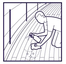
Prepare the surface with Q<sup>2</sup>R Degrease. Use a moderate amount of product and wipe with a microfibre. Ensure the surface is oil free and completely dry.
